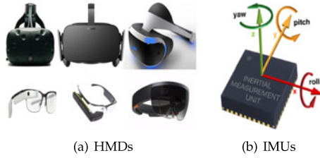
Fig. 1. Left: Examples of AR/VR headsets in the market; right: IMUs and its axes.
